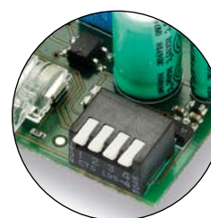
SENSITIVITY SELECTION DIP-SWITCHES
