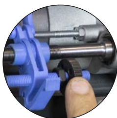
INTEGRATED OPENING AND CLOSING TRAVEL LIMITS
