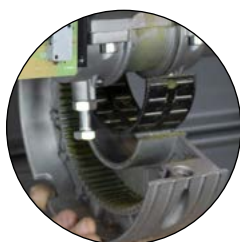
CROWN WHEEL MOUNTED ON ROLLER BEARINGS
