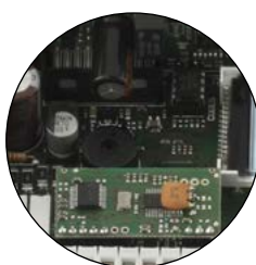
433MHz OR 868MHz INTEGRATED RECEIVER CARDS
