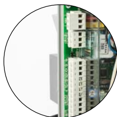
ELECTRONIC PROGRAMMER WITH EXTRACTABLE TERMINAL BLOCKS
