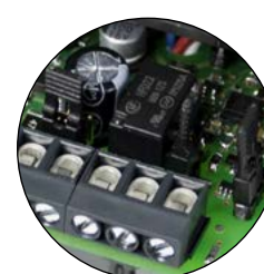
RELAY OUTPUT SELECTION N.C.-N.A. OR 8,2KΩ USING JUMPERS.
