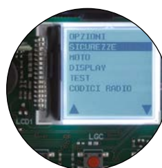
SELF-PROGRAMMING MONITORED BY AN LCD GRAPHICS DISPLAY
