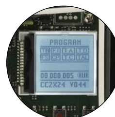
SELF-PROGRAMMING MONITORED BY AN LCD GRAPHICS DISPLAY VERSIONS HL2524ESB - HL1824ESB
