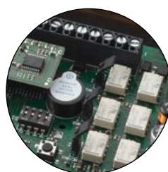
STATIONARY TRANSCEIVER, SAFETY OUTPUT MANAGEMENT (NO/8,2kΩ)
