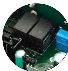
DOUBLE RELAY WITH SERIAL EXCHANGE NO-NC
