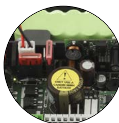
EMERGENCY NiMH BATTERIES IN THE CC242ETOPCB AND CC242EXTOPCB VERSIONS
