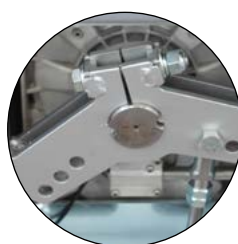
REINFORCED BALANCE SYSTEM AND GEARED MOTOR PERSONALISED FOR THE 3,4,5 METRE BOOMS OF THE ELDOMSDG
