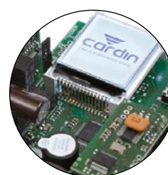
SELF-PROGRAMMING MONITORED BY AN LCD GRAPHICS DISPLAY
