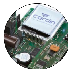
SELF-PROGRAMMING MONITORED BY AN LCD GRAPHICS DISPLAY
